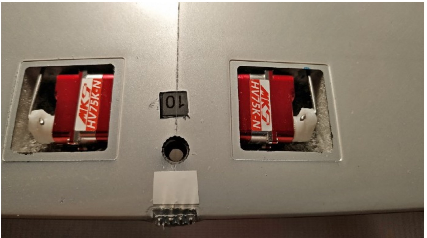
Photo 6: The aileron servos in place, just glued with rapid epoxy.
