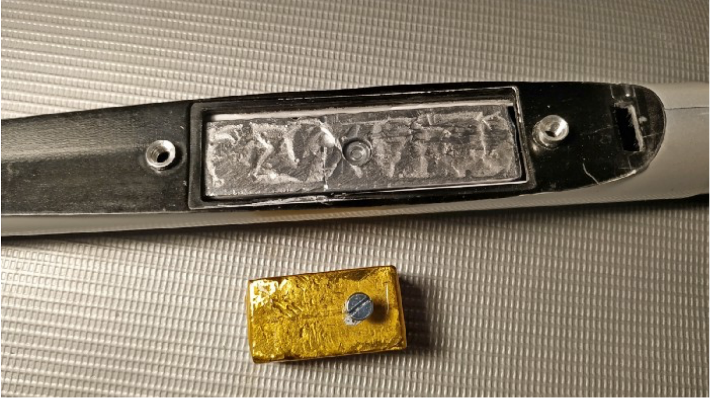
Photo 8: The two ballasts, 85gr for the smallest and 190gr for the heaviest. It is possible to go further with a 2 pieces ballast
