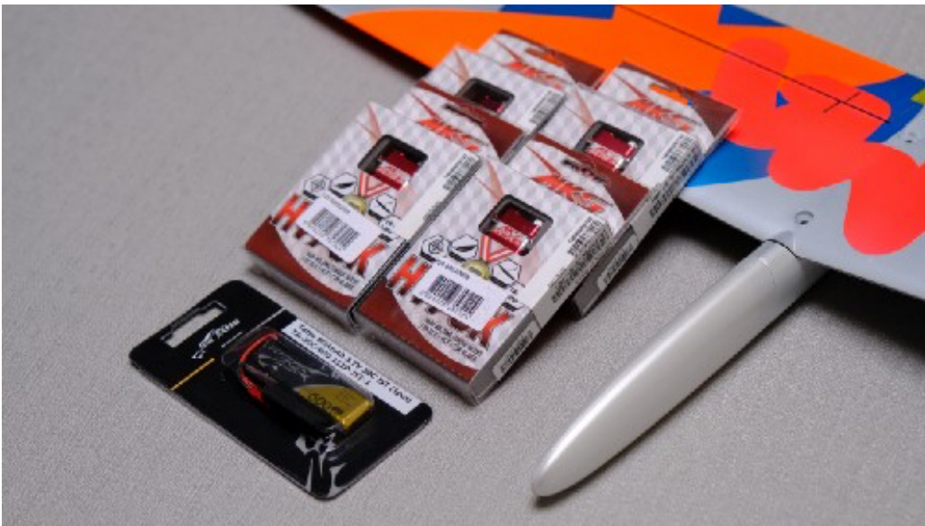
Photo 3: 4 MKS HV75K-N servos and 1s LiPo battery.
